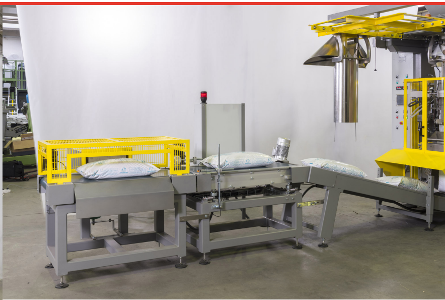
Stainless Steel Form/fill/seal machine Mod. CV4025 with weighing unit
